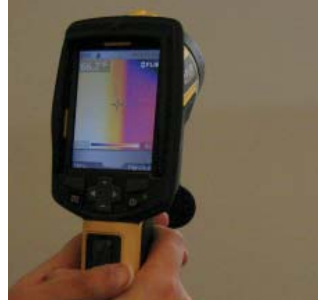
Sigma's infrared moisture detector
